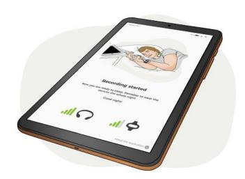
The tablet delivered with the Nukute sleep apnea measurement system is the primary source of user instructions. Tablet is used as a router, it receives measurement data from neckband and send it to cloud for analysis.
