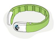
There are four different size neckbands inside the carrying case (X, S, M and L). Measurement and battery modules are needed when using neckband. Assembled neckband is used for recording breathing sound and detecting sleeping position. Measurement module contains microphones for breathing sound measurement and a motion sensor for sleeping position definition.
